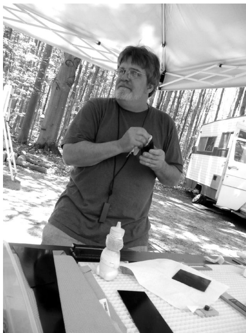
Joe Smigiel polishing glass plate with a calcium carbonate solution.
