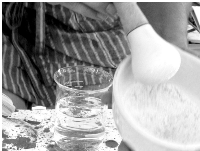
Gum Sandarac nuggets are crushed in mortar for making varnish.
