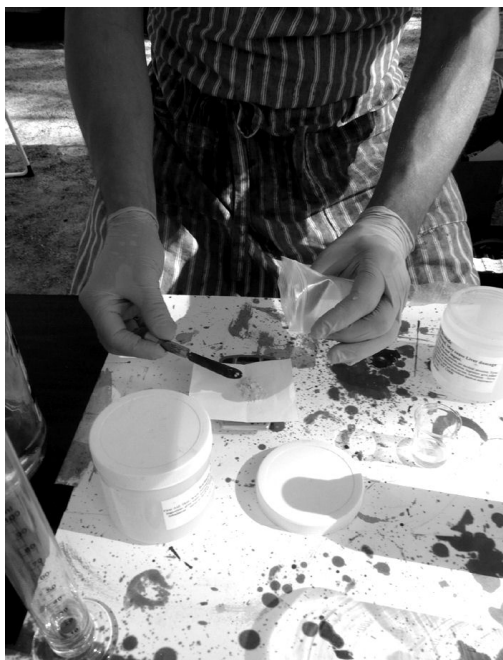
Bill Schwab measuring cadmium bromide that when in solution with potassium iodine and distilled water will be mixed with a solution of collodion USP diethyl ether and grain alcohol for the resulting salted collodion solution.
