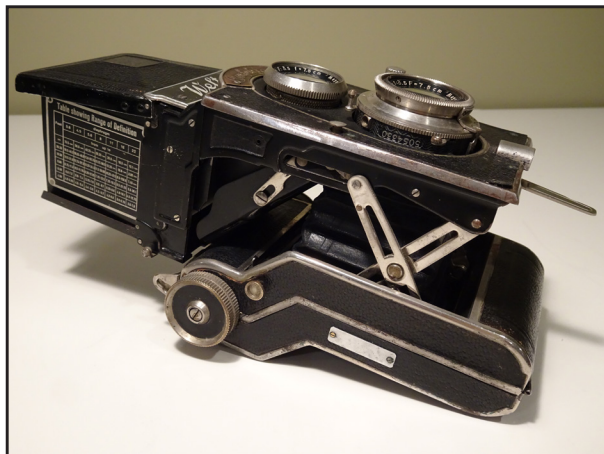
The Perfekta in shooting position showing lazy struts and mirror and viewfinder in open position. It has auto stop film advance but no double exposure prevention.
