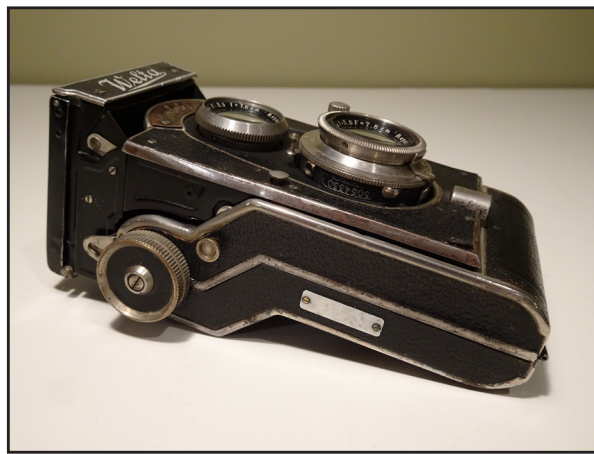
The Perfekta in its collapsed state which reduces the depth of the body by about 1 1/2 inches. Although the mirror collapses, the viewfinder glass does not, which limits the advantage of this function somewhat.
