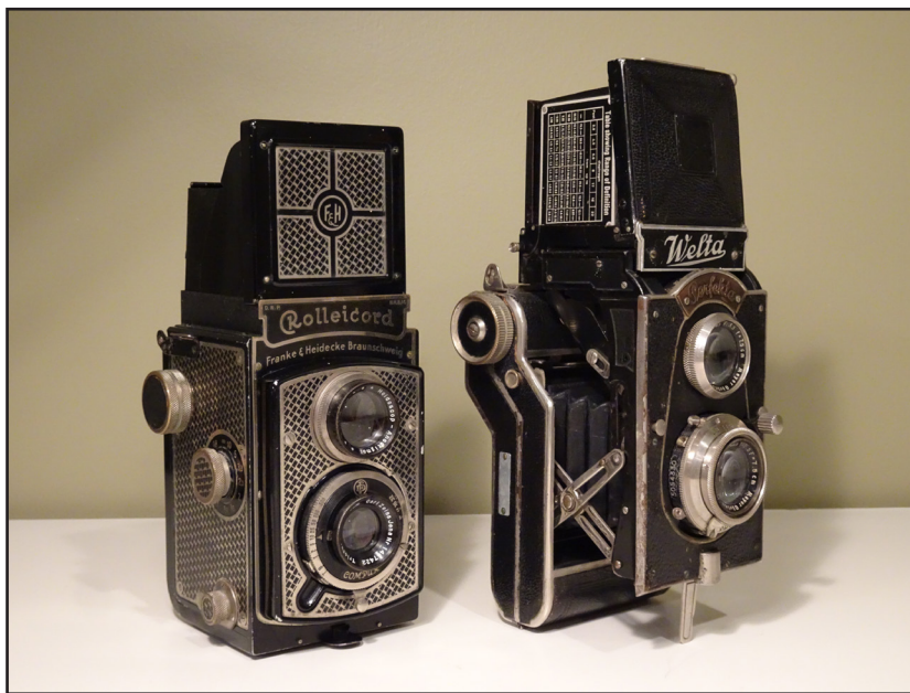
This shows the relative size of the Perfekta compared to a standard TLR of its day. The weights are comparable due to the extensive use of aluminum in the more complex Welta body compared to the Rolleicord's mostly brass body.
