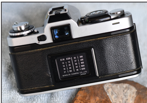
The back of the XD-11. There was a slot to place an end of a 35mm film box to remind the photographer of the film loaded in the camera. Very useful when a film was loaded for an extended length of time before it was ready for processing.
