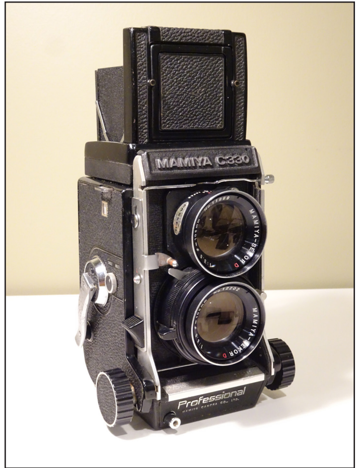
The Mamiya C330 and its lineage was produced from 1957 until 1983 mainly as a professional studio camera, but was rugged enough to be used in the field. Its main attribute was its excellent interchangeable lenses mounted on bellows allowing closeups as near as 7 inches without accessories. Shown here with standard waist-level viewfinder.
