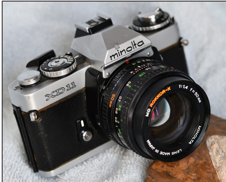
This magnificent Minolta XD-11, which set a new standard for SLRs—allowing photographers three choices for making pictures: full manual control, aperture preferred shooting, or shutter preferred. The behind-the-lens shutter was also electronically controlled.
