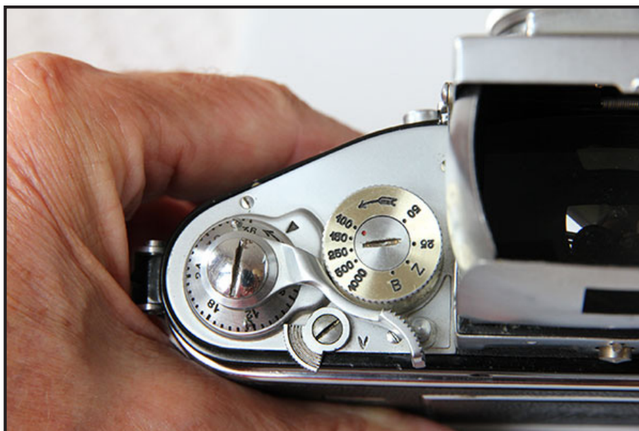
Old-fashioned rotating lift-and-turn shutter dial and ultra-long throw left-handed film advance. Not the last word in convenience.
