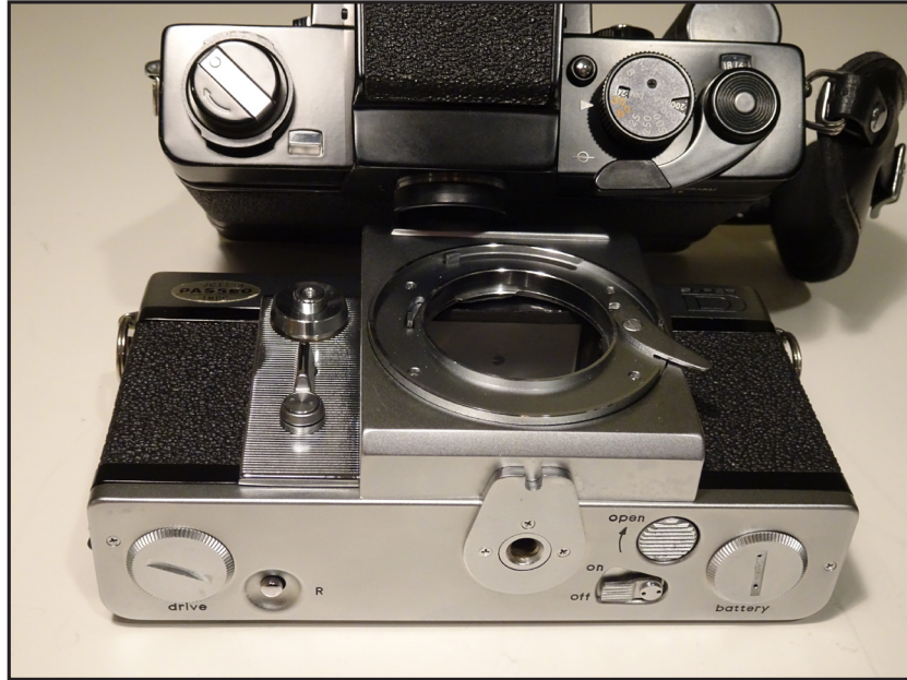
View showing all Super D controls. Bottom includes drive linkage port, rewind button, meter switch, film back push button and battery chamber. Above includes film/shutter speed dial and film advance lever. Face includes shutter release button above delayed shutter control. Notice Exakta bayonet lens mount and trigger lock.
