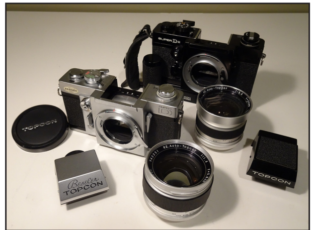
Exploded view of the Topcon Ds showing removable pentaprisms, 5.8cm lens (front) and 25mm lens. The film winder motor does not appear to be removable from the black Dm body.
