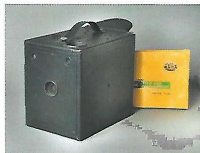
4x5 Eastman Kodak Premo Jr. No. 4 which has interesting film pack on back 1909-1914
