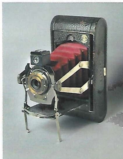
No 1A Folding Pocket Kodak camera with red bellows, twin spring struts, 1905-15
