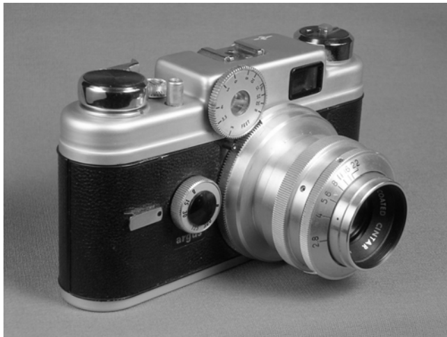
C4R camera. The C4R incorporated “rapid” film advance and rewind, as well as an integrated light meter that mounted on the shoe seen on the right front of the camera.
