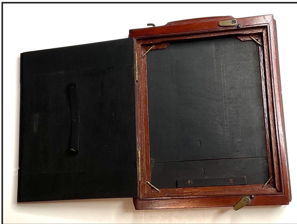
Wet collodion plate holder with open door and showing a wire at each corner on which the plate rests.
