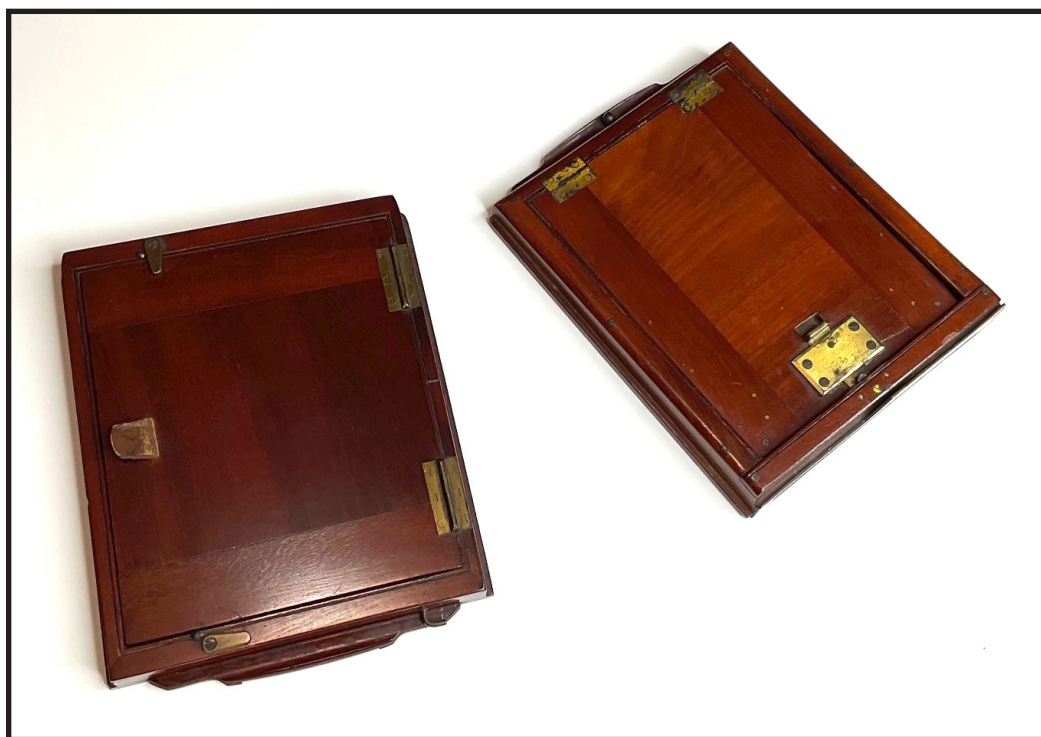
(Left) Wet collodion plate holder with leather tab and two hinges. (Right) Dry plate changing slide showing the brass connector that attaches to the changing box. Note the trapezoidal shape of the longer side.
