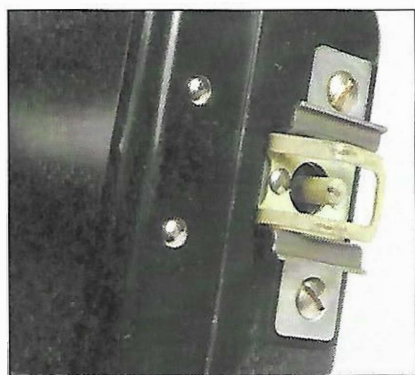
Model 21's flash used a bulky accessory shoe bracket with a large center probe.
