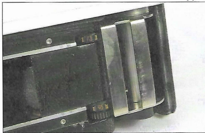
A film guide device was used until serial number 20000 because the advancing film cocked the shutter in the early units.
