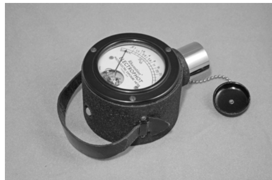
FIGURE 11. The Model DH is real hefty for an exposure meter weighing in at one pound, 3½ ounces without its two AA batteries and is 3½ inches in diameter and 2½ inches thick. The snout serves to keep stray light off the cell in order to cover the same area as a normal lens.
