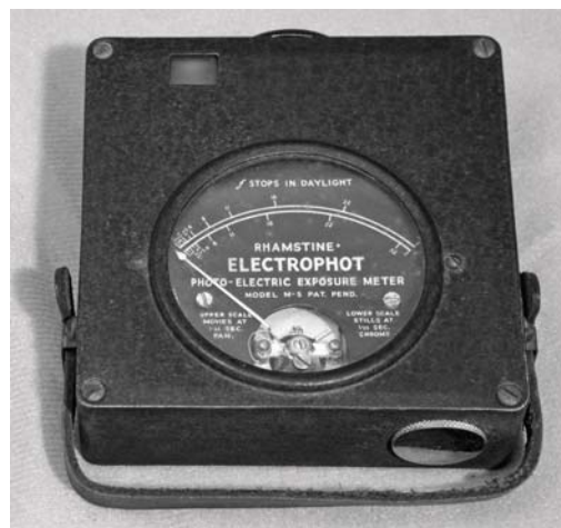
FIGURE 15. At the lower right of the Model MS is the cover to the battery compartment but batteries were not longer required.
