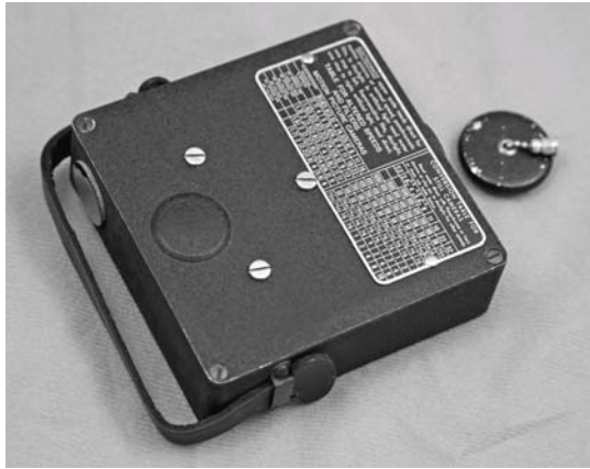
FIGURE 17. The underside of the Model MS has tables for different camera speeds and a table for still camera use. The plug is to protect the cell when the meter was not in use.
