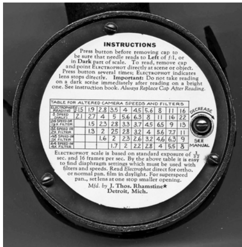
FIGURE 12. Instructions are on the backside of the Model DH meter along with a table for different frames/second camera speeds and filters. The cautionary points are just like those for cadmium sulfide cells introduced in 1960.
