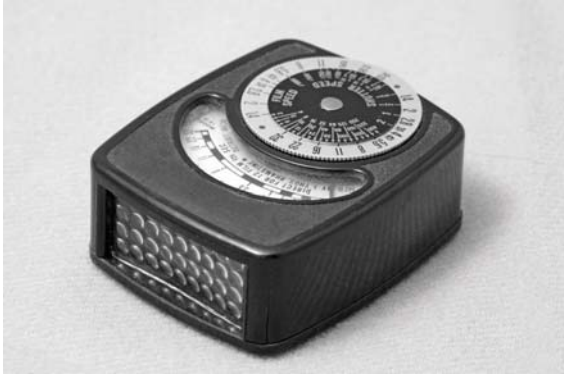
FIGURE 21. The revised Model 14A can be distinguished from the prewar Model 14A by the Electrophot name being on the dial scale and the plastic multilens cover over the cell.
