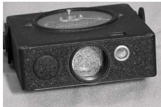
FIGURE 16. The "Rhamstine Electronic Cell" in the Model MS has the shiny appearance of galvanized zinc. To the right is the viewfinder.
